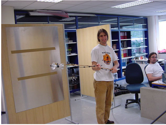
Figure A-15: "Schwenkmethode" with biconical antenna (2)
