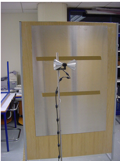
Figure A-10: Measurement with biconical antenna
