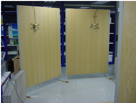
Figure A-9: Planar antennas setup
