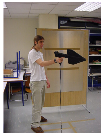
Figure A-18: "Schwenkmethode" with directional antenna (3)
