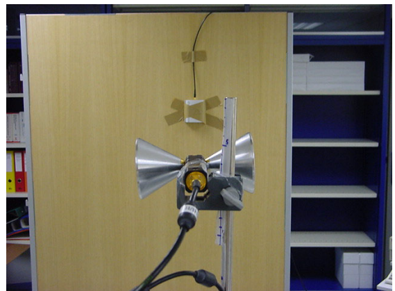
Figure A-13: Biconical antenna polarization
