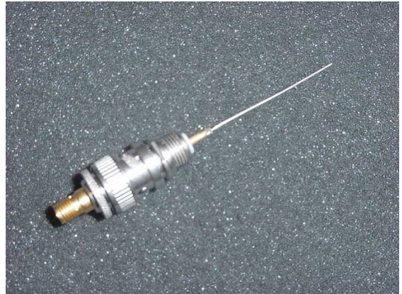
Figure A-6: Wire antenna \lambda/4
