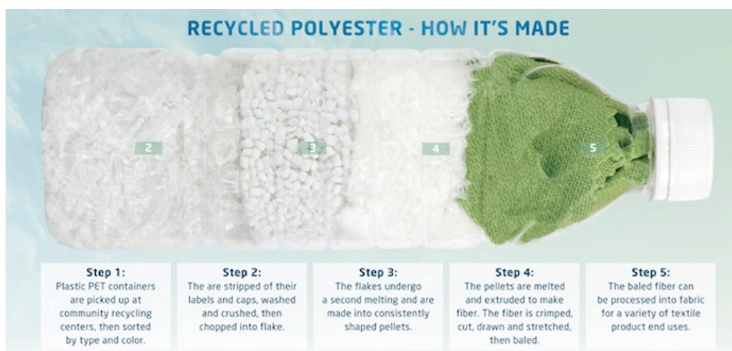
Figure 6: Visual representation of the process to make recycled polyester fiber from PET bottles
