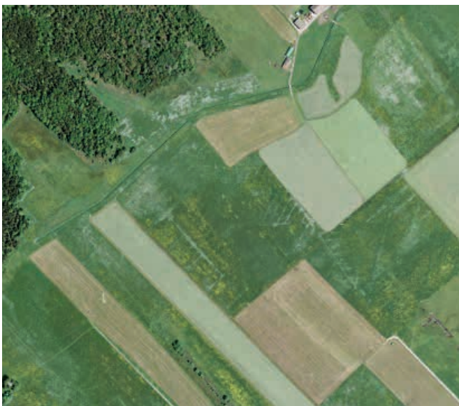
Fig. 38 Agricultural drainage can be clearly seen from a bird's eye view.
