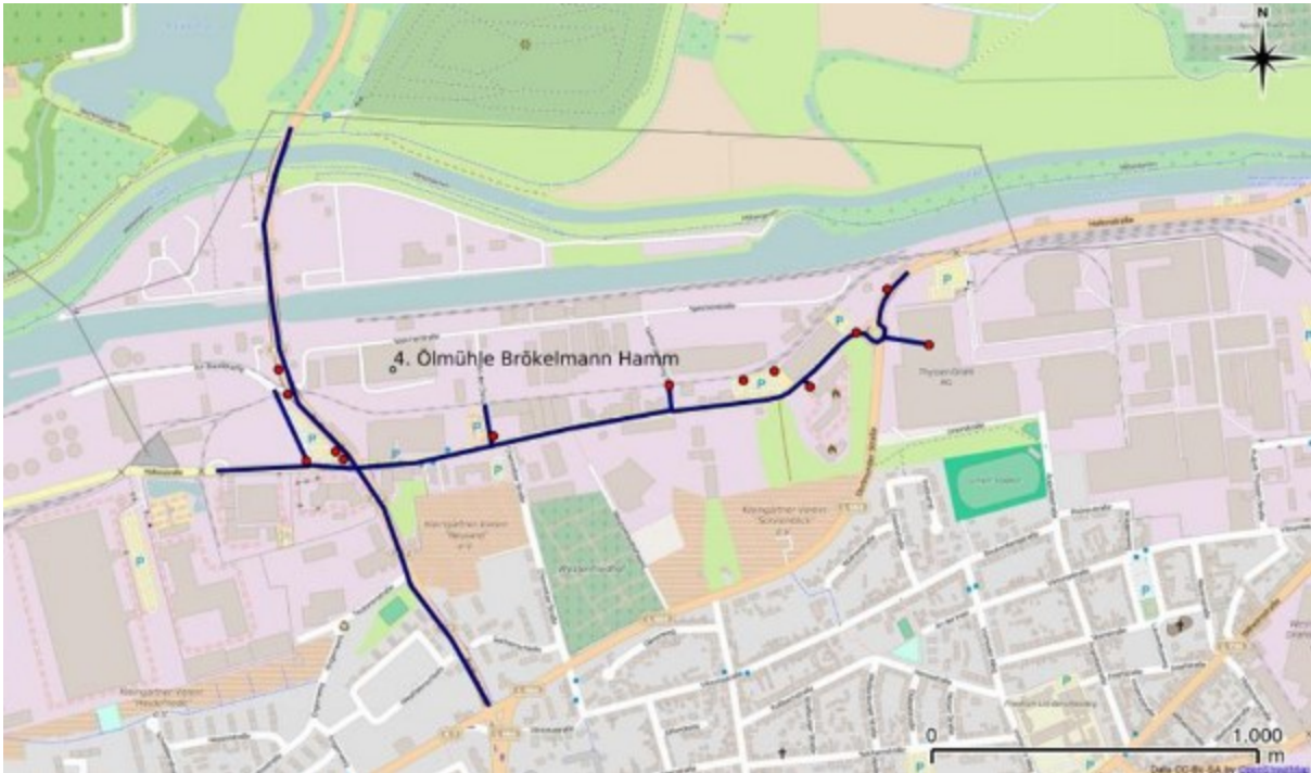
Fig. 9: Sampling locations (red dots) including survey tracks (tracks in dark blue) in Hamm near to the oil mill of Brökelmann Co. Ölmühle GmbH & Co.. The road, rail and waterway networks are also visible. By no means all the access roads and railway tracks were actually surveyed. Plan produced in QGIS 2.2.0 using Openstreetmaps as the base map. After Wedlich et al. (2016).
