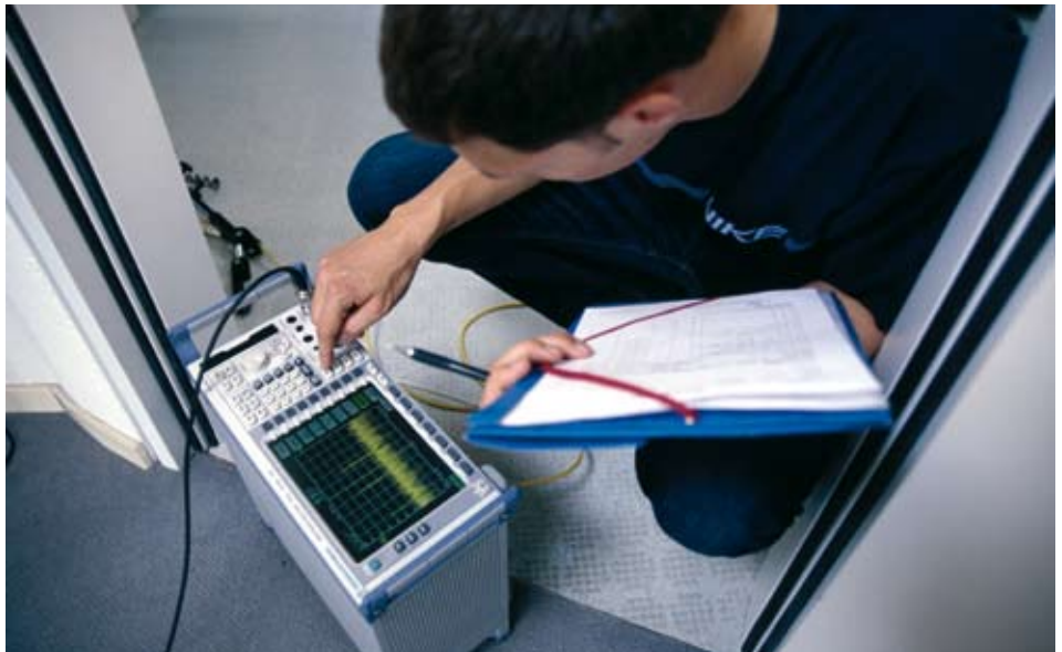
This hand-held test antenna (above) can be used for detecting the maximum exposure level indoors. A spectrum analyser (below) depicts the results of the frequency selective measurement. Since each frequency is recorded separately, it is possible to specifically measure the level of radiation from a single mobile phone base station.
