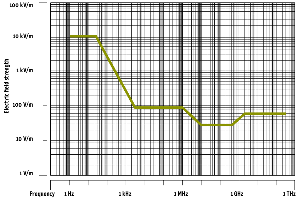
The exposure limit values for the electric field strength (green curve) specified in the ONIR vary according to the frequency of the radiation, since the effects on human beings occur at different intensities depending on frequency.
