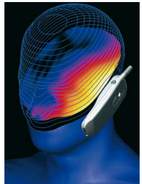
Example of the calculation of radiation exposure of the head when using a mobile phone: the model concerned has an SAR of 0.61 W/kg. The highest exposure is in the white/yellow zone in the outer layers. The exposure diminishes rapidly towards the interior. In the black zone it is 100,000 times weaker than in the outer layers. (Original image from IT'IS Foundation, Federal Institute of Technology, Zurich)
