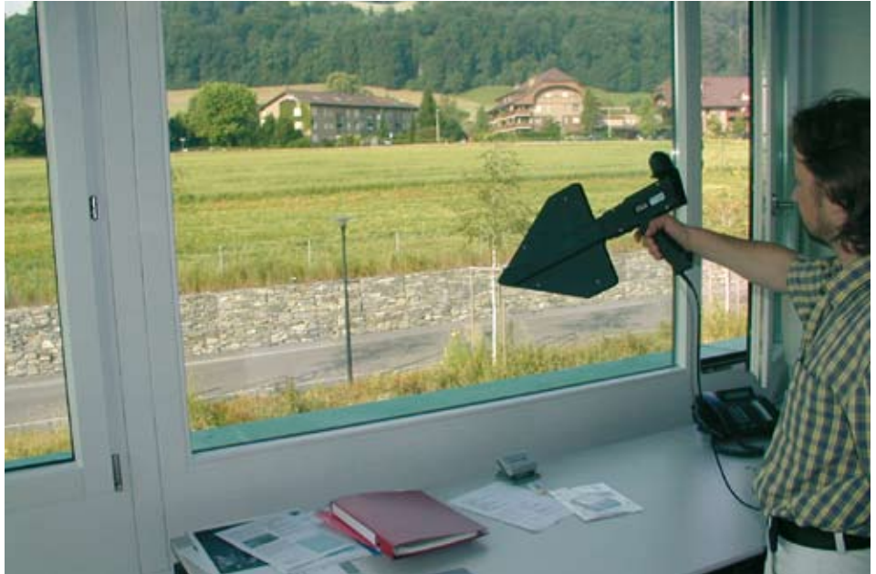
This hand-held test antenna (above) can be used for detecting the maximum exposure level indoors. A spectrum analyser (below) depicts the results of the frequency selective measurement. Since each frequency is recorded separately, it is possible to specifically measure the level of radiation from a single mobile phone base station.
