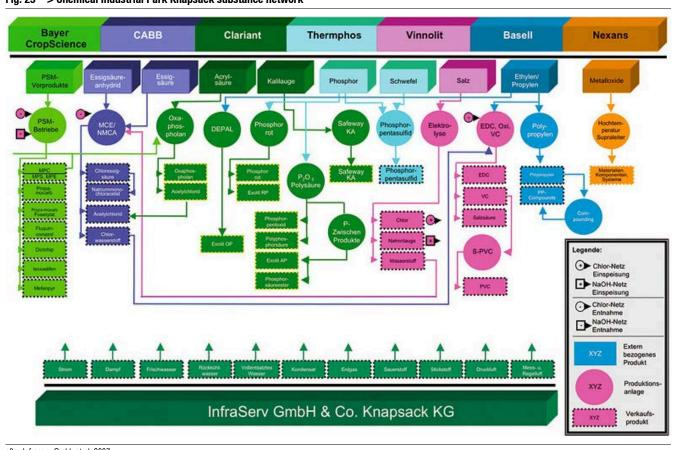
Fig. 23 > Chemical Industrial Park Knapsack substance network
