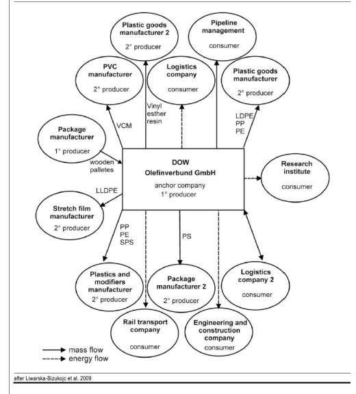
Fig. 24  $\,$  > Aerial view of the material flow scheme of the main symbiotic relationships between the fourteen companies at the Dow Value Park
