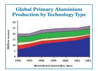
As a result, older Horizontal Stud Søderberg (HSS), Vertical Stud Søderberg (VSS) and Side Work Prebake (SWPB) technologies represent an ever smaller proportion of global production.
