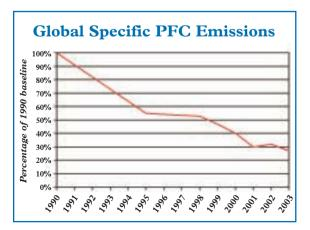
Much of this reduction is due to the phasing in of new Point Fed Prebake (PFPB) and Centre Work Prebake (CWPB) plants.
