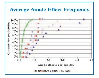
The above Anode Effect Frequency graph highlights not only the significant difference in performance between modern PFPB and other technologies, but also the wide spread of performance within all the technology categories. There is also
