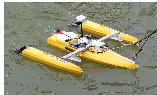
Acoustic Doppler current profiler on a trimaran. Photo: Beat Sigrist
