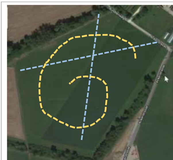
Fig. 1: Soil sampling according to ÖLN methodology. 20 samples are taken (blue: along two crossing lines, or yellow: randomly distributed).
