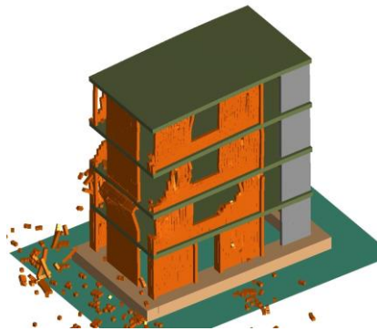
Figure 13: Collapse of the model during test 6 (PGA=0.6g)
