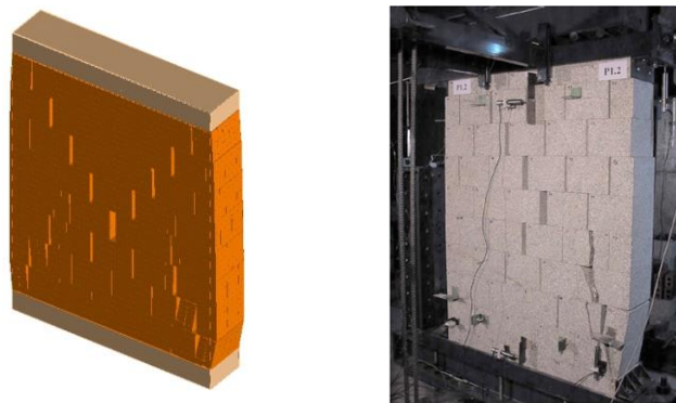
Figure 7: Comparison of damage in the AEM model and the experimental test for the in-plane cyclic loading
