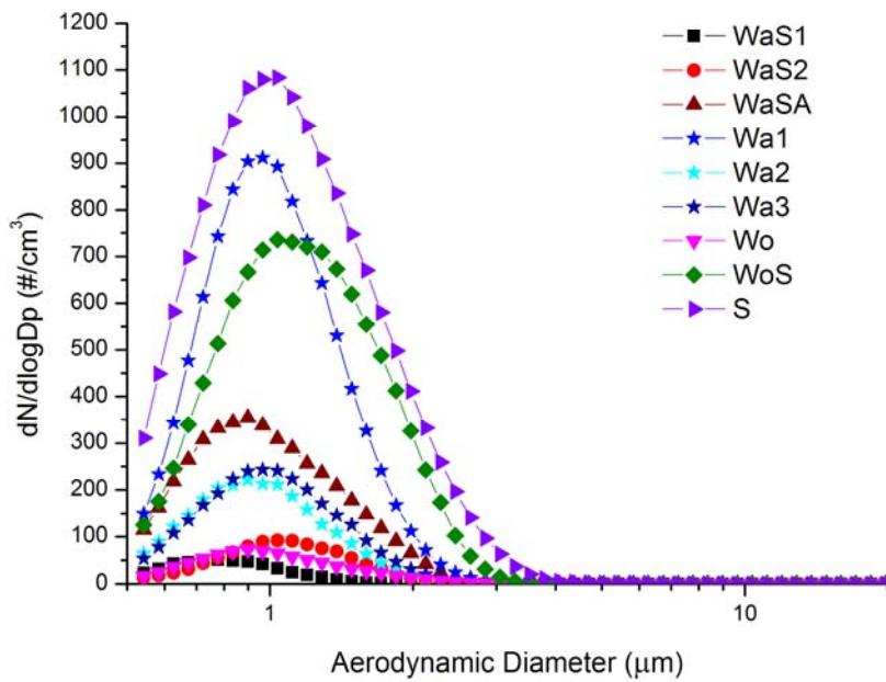
*Fig. 17: APS results for all the fly ashes (named as listed in Tab. 2). The size range covered by APS ranges from 0.5 and 20  $\mu\text{m}$ .*
