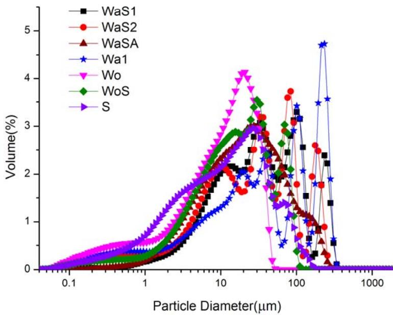
*Fig. 14: Laser Scattering (LS) analysis of the fly ashes before the fractionation; volume percentage.(mass based result)*
