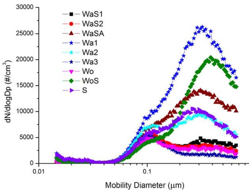
*Fig. 16: SMPS results for all the fly ashes (named as listed in Tab. 2) for the size range between 0.015 and 0.7  $\mu\text{m}$*
