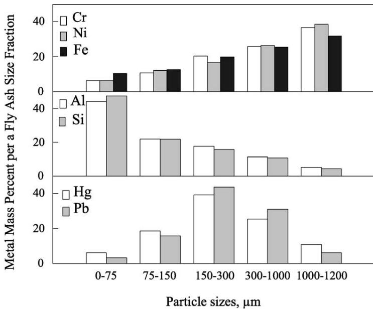
*Fig. 10: Chemical composition as mass percentage of different size fractions in fly ash from a lab scale municipal waste incinerator [48].*
