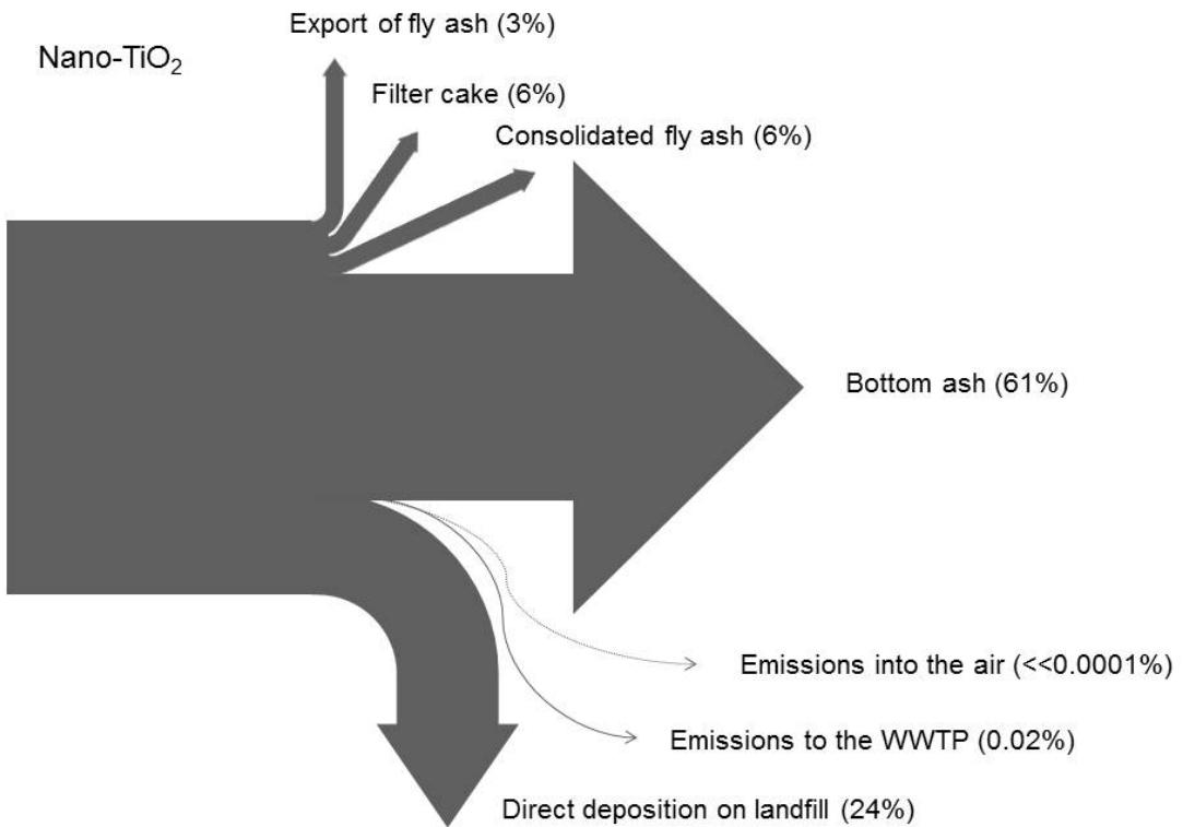
Fig. 24: Waste disposal as input-output system for nano-TiO<sub>2</sub>. Total input: 155 t/a
