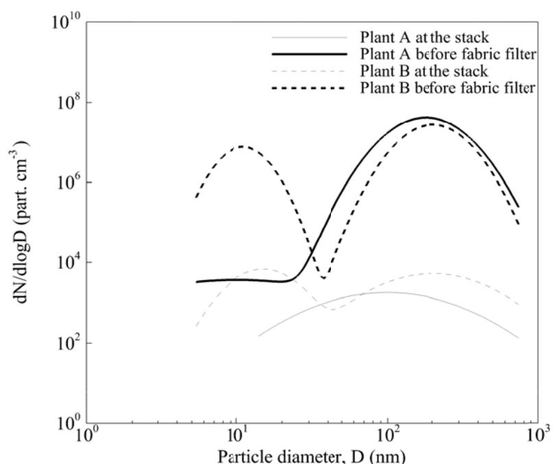
Fig. 6: Measurements of the particle emissions from a waste incineration plant [45].
