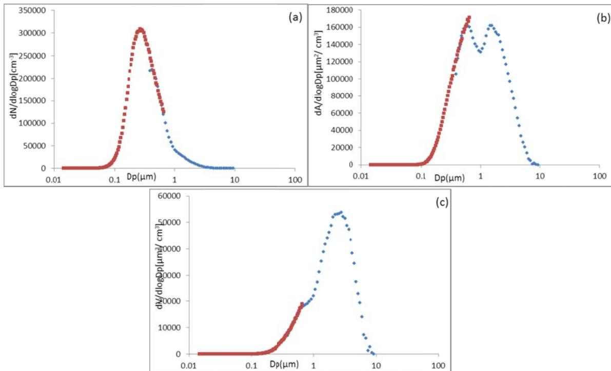
*Fig. 20: Illustration of the merging routine. The final optimum fitting is included for (a) number, (b) surface area and (c) volume representations for TiO<sub>2</sub> SR 2400 sample.*
