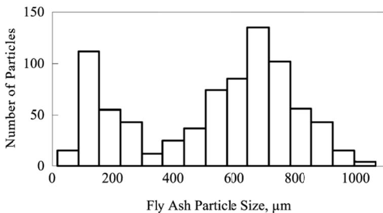
Fig. 8: Size distribution (particle number) of the fly ash particles from a lab scale municipal waste incinerator determined using optical microscopy. The first bar in the graph represents the fraction of particles between 0-75  $\mu\text{m}$  [48].
