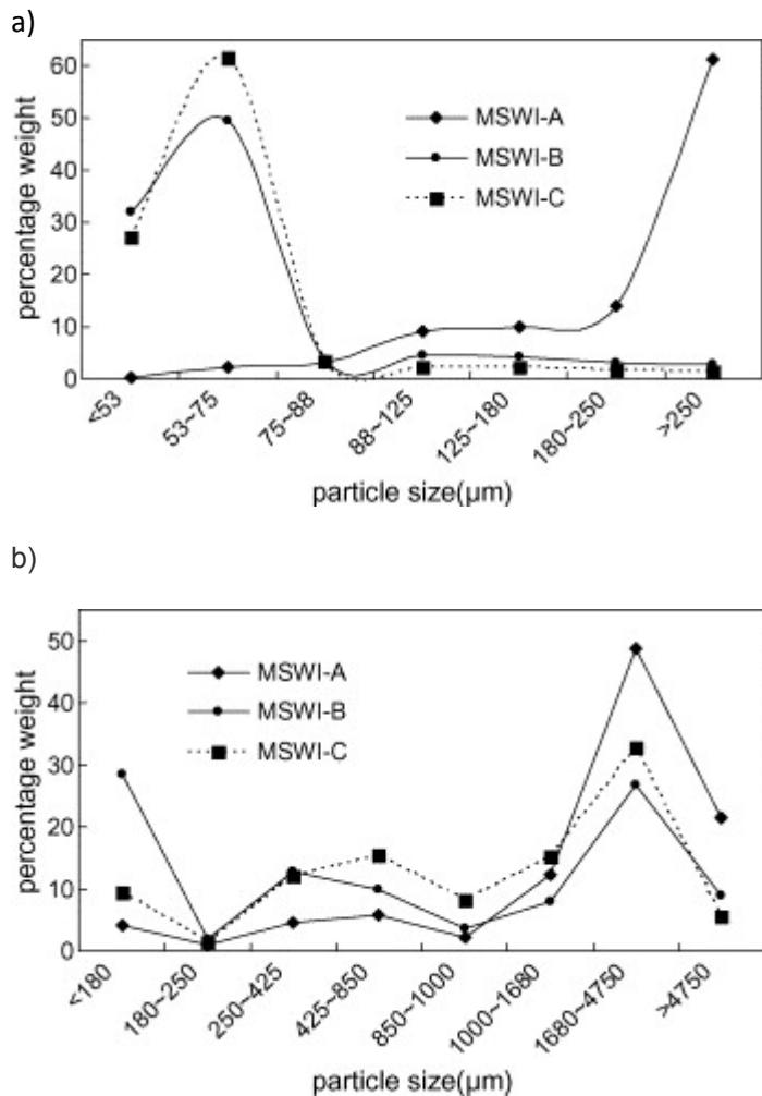
Fig. 7: Particle size distribution given as percentage of weight (a) in fly ash and (b) in bottom ash from three municipal solid waste incinerators [46].
