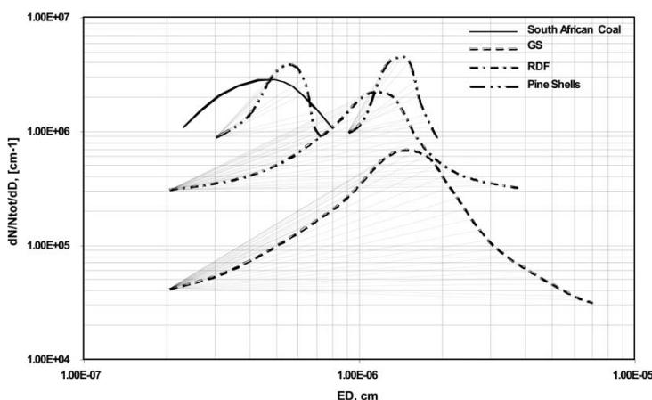
Fig. 4: Particle size and number concentration of ultrafine particles in the exhaust of an experimental fluidized-bed reactor after a high efficiency cyclone with four different fuel types: South African bituminous coal, GS (commercial predried granulated sludge), RDF (refuse derived fuel) and pine shell (biomass waste). ED reports the equivalent diameter of a sphere of equal volume. [36]
