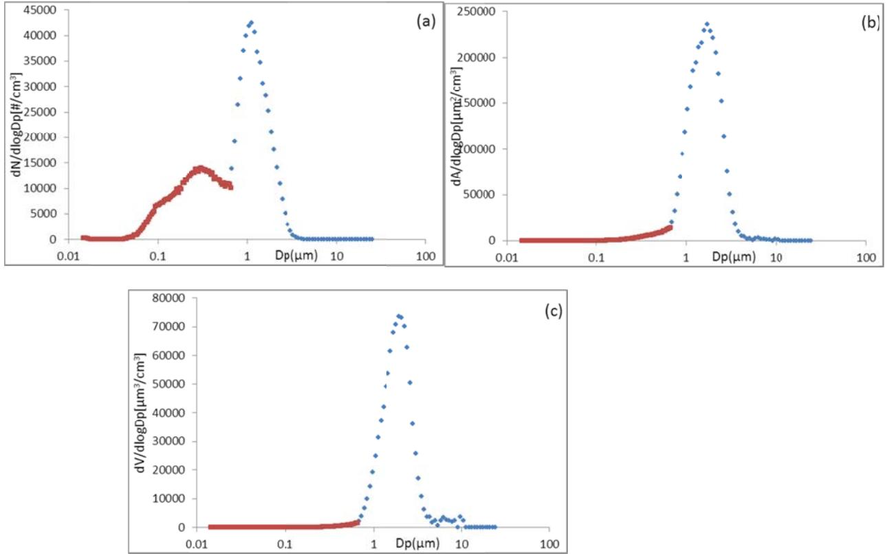
*Fig. 18: Fitted spectrum of the SMPS and APS results according to merging data routine. The final optimum fitting results are presented for (a) number, (b) surface area and (c) volume for the fly ash sample WaSA.*
