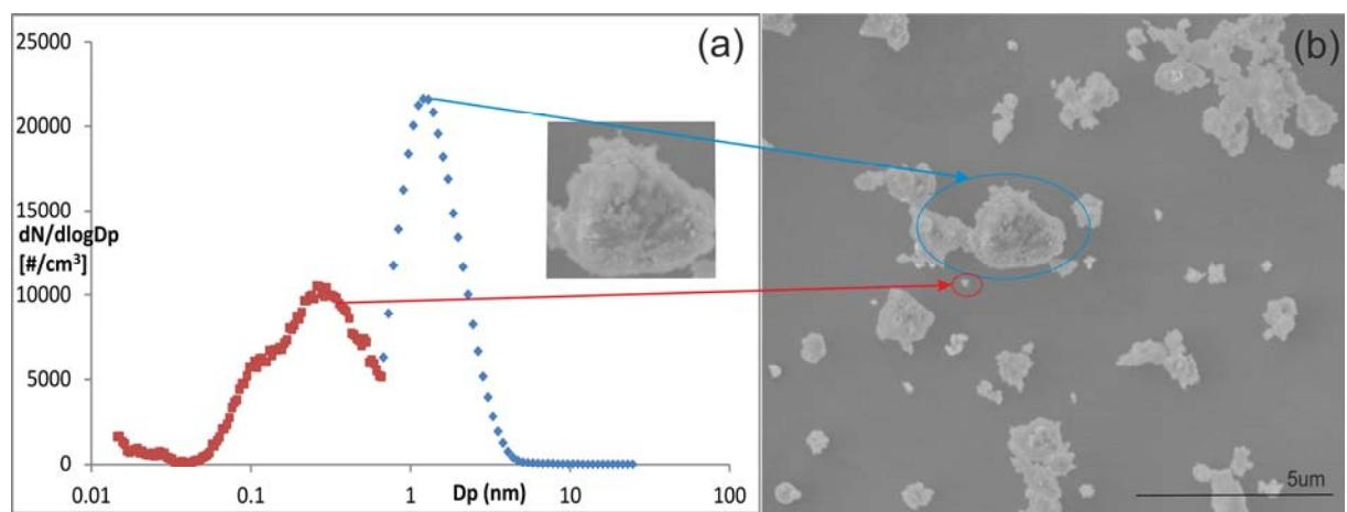
*Fig. 32: Sample S - size and morphology analysis (a) Fitted spectrum of the SMPS and APS results according to merging data routine; (b) SEM image showing smaller (highlighted in red) and bigger (highlighted in blue) ash particles, in good correlation with sizes measured.*
