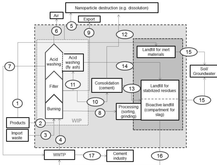
Fig. 21: Generic model describing the waste disposal system in Switzerland focusing on waste incineration and landfills. WWTP: waste water treatment plant, WIP: waste incineration plant.
