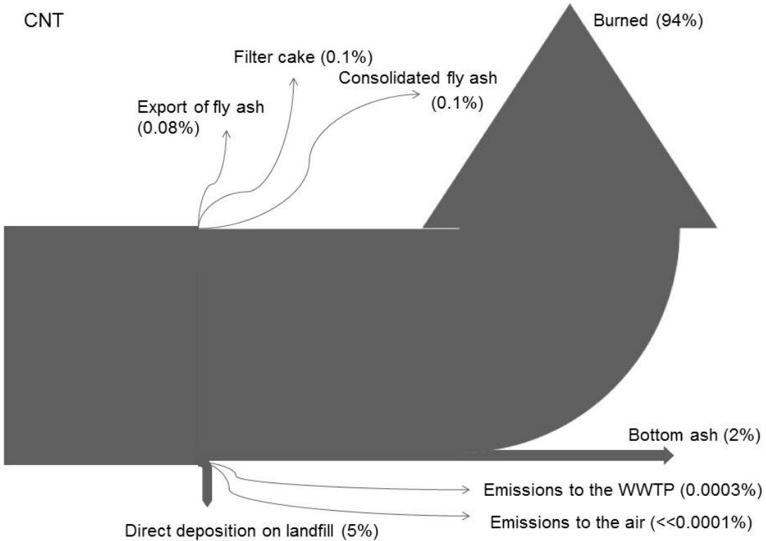
Fig. 30: Waste incineration as input-output system for CNT. Total input: 1.36 t/a. The difference to 100% is due to rounding.
