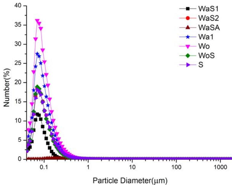
*Fig. 15: Laser Scattering (LS) analysis of the fly ashes before the fractionation; number percentage.*
