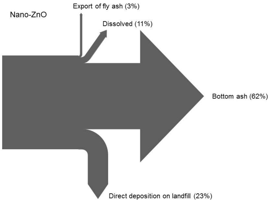
*Fig. 26: Waste disposal as input-output system for nano-ZnO. Total input: 5.55 t/a. The difference from 100% is due to rounding.*
