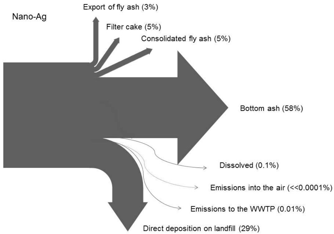
*Fig. 28: Waste disposal as input-output system for nano-Ag. Total input: 1.18 t/a*
