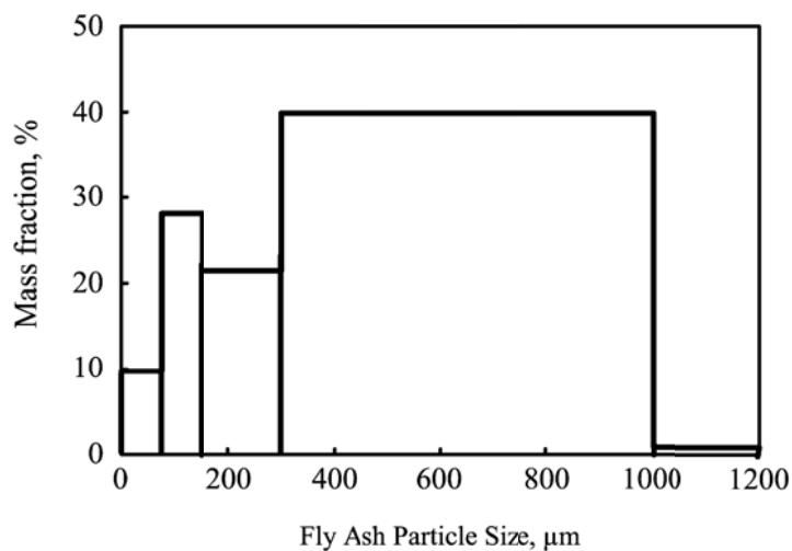
Fig. 9: Size distribution as mass fraction in weight percent (wt-%) of the fly ash particles from a lab scale municipal waste incinerator determined using sieving. The first bar in the graph represents the fraction of particles between 0-75  $\mu\text{m}$  [48].
