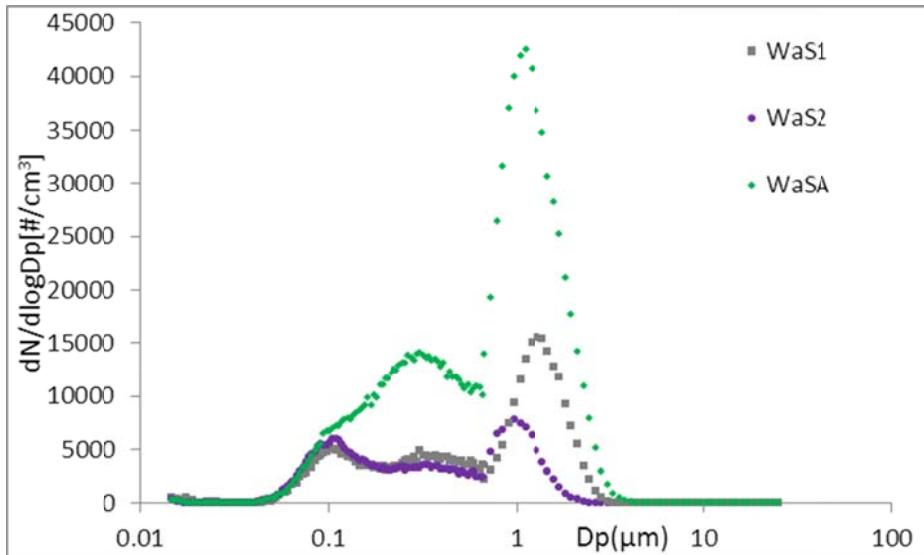
*Fig. 19: The final optimum fit for number representations of SMPS and APS spectrums merged for WaS1, WaS2 and WaSA fly ashes.*
