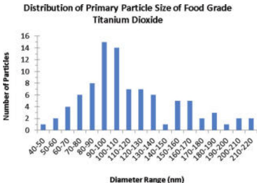
Fig. 12: Particle size distribution of food-grade TiO<sub>2</sub> [28]
