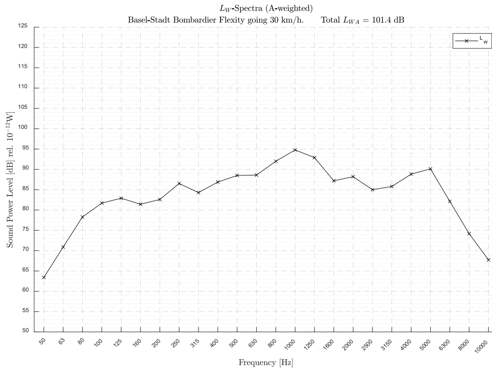
Figure 34: Sound power level spectrum of a Bombardier Flexity (Basel) tram going 30 km/h
