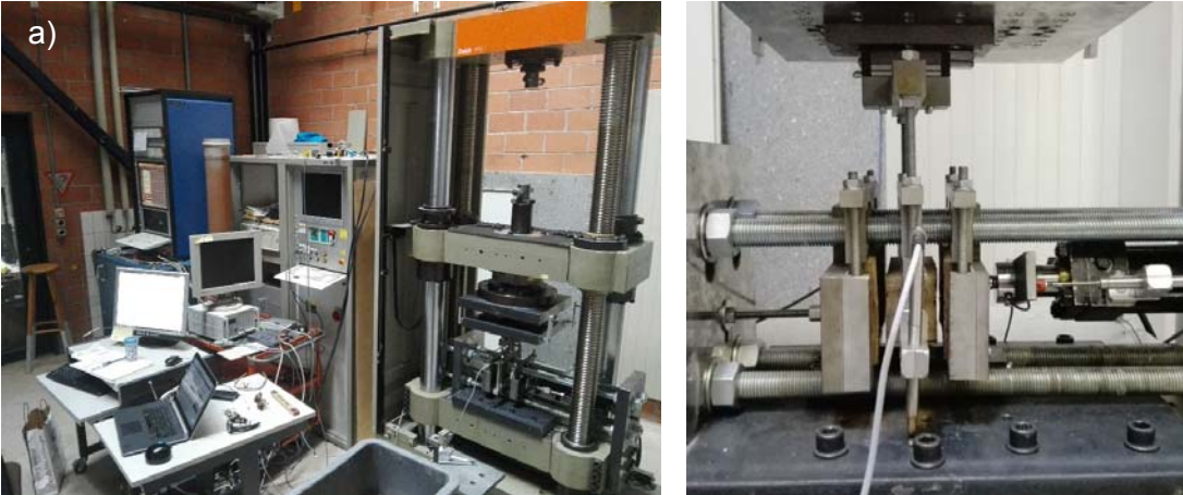
Figure 3 (a) Overview of the test setup, with double-actuator testing machine on the right-hand side, control system on the left, and data acquisition software in the centre; (b) Close-up view [8].
