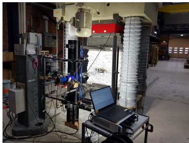
Figure 7 Test setup and instrumentation used for the pull-out tests: photo [15].
