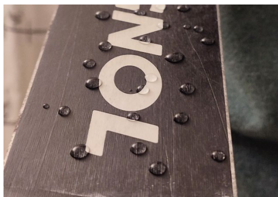
Fig. 1: Water droplets beading on a surface treated with fluorinated wax [2].
