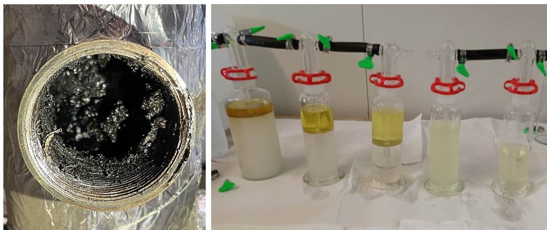
Figure 18: Plastic gasification. Left: Raw gas duct section of a gasifier after gasification of plastic waste, right: Scrubbing bottle battery for cleaning a partial gas stream of this gasifier before analysis. (Photo: C. Schmittmann).
