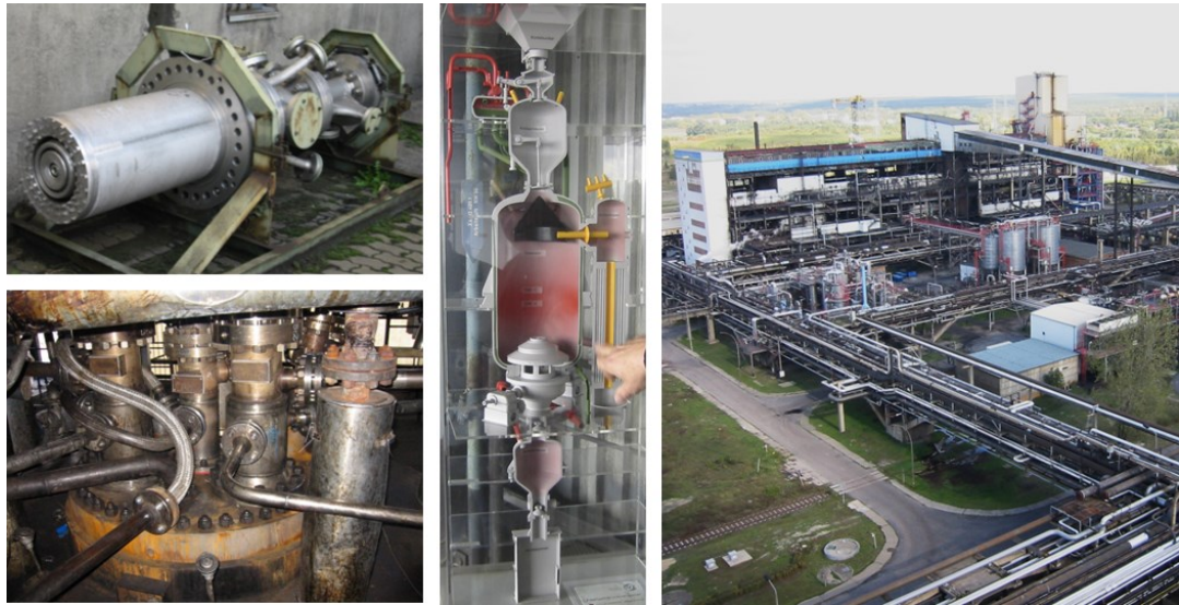
Figure 10: Gasification infrastructure at SVZ Schwarze Pumpe, Germany (2003). Left: Oil-steam burner nozzle and reactor head of entrained flow gasification, middle: model of entrained flow gasifier, right: gasifier building with 6 fixed bed reactors.
