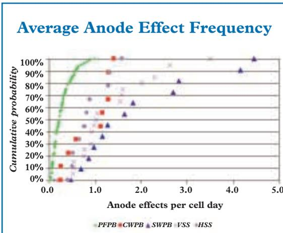
The above Anode Effect Frequency graph highlights not only the significant difference in performance between modern PFPB and other technologies, but also the wide spread of performance within all the technology categories. There is also
