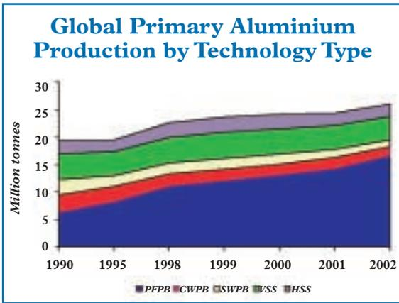
As a result, older Horizontal Stud Søderberg (HSS), Vertical Stud Søderberg (VSS) and Side Work Prebake (SWPB) technologies represent an ever smaller proportion of global production.
