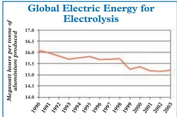
As well as reducing specific emissions of PFCs, by 73% per tonne of aluminium produced, progress towards good practice and investment in modern technology has also contributed to a 6% drop in smelting energy use since 1990.
