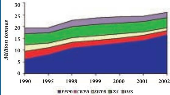
As a result, older Horizontal Stud Søderberg (HSS), Vertical Stud Søderberg (VSS) and Side Work Prebake (SWPB) technologies represent an ever smaller proportion of global production.
