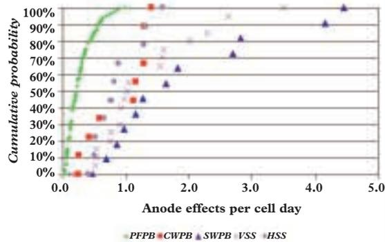
The above Anode Effect Frequency graph highlights not only the significant difference in performance between modern PFPB and other technologies, but also the wide spread of performance within all the technology categories. There is also
