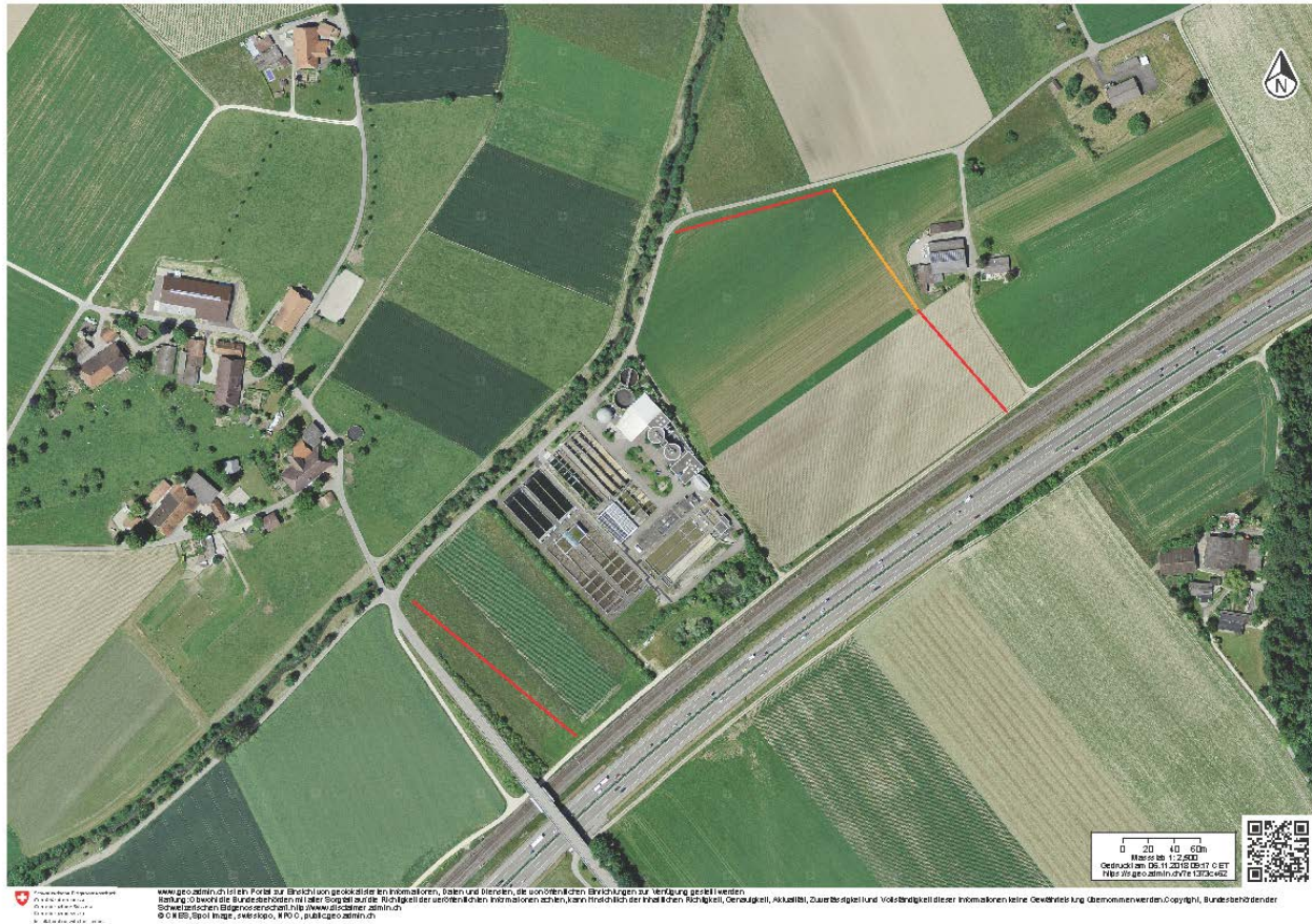
Figure 4: WWTP Moossee-Urtenenbach and its surrounding area. Prevailing wind direction: west, south-west. The red and orange lines indicate the approximate position of the line integrated measurement devices.
