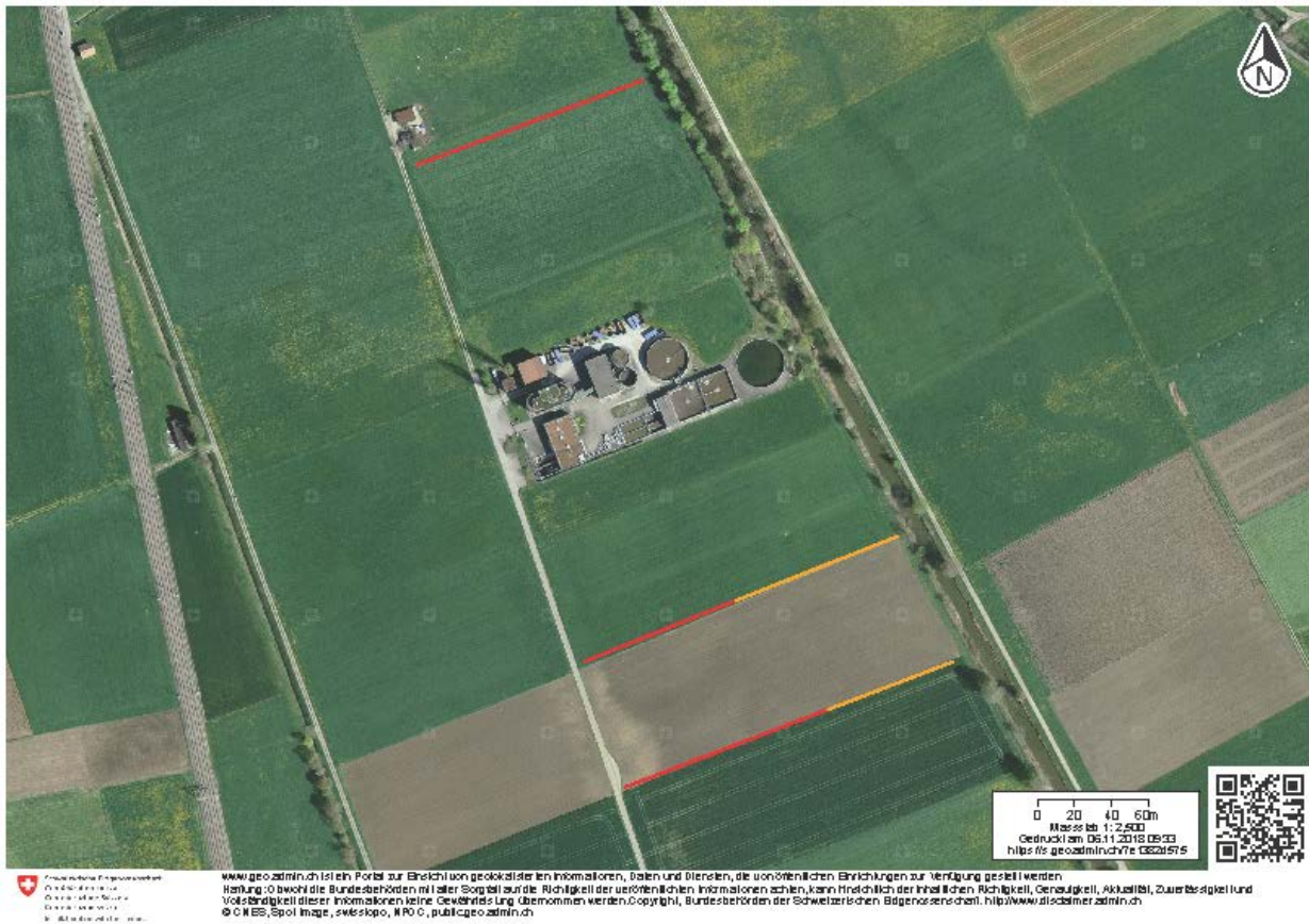
Figure 5: WWTP Gürbetal and its surrounding area. Prevailing wind direction: north, north-east. The red and orange lines indicate the approximate position of the line integrated measurement devices.
