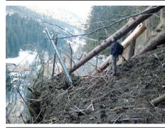
**Damage** Tree impact on a net barrier
