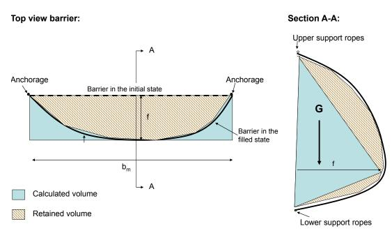
Fig. 24. Net deflection and self-weight of the net's belly. Figure according to [36].
