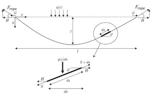
Fig. 13. Representation of the rope equation for equal load on the deflected rope, according to [20] and [36].
