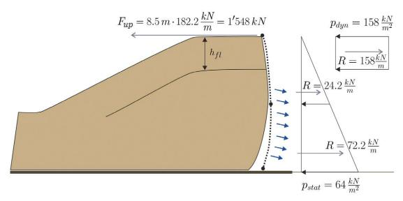
Fig. 23. Last pressure surge flowing into the protection net before the overflow begins. Decisive case for the calculation of the upslope anchor ropes.
