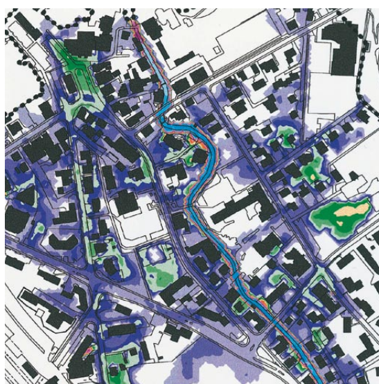
Figure 7: Intensity map: It shows the intensity for a selected recurrence period of 30, 100, or 300 years as well as for an extreme event. This information is of importance in assessing flood-proofing measures.
