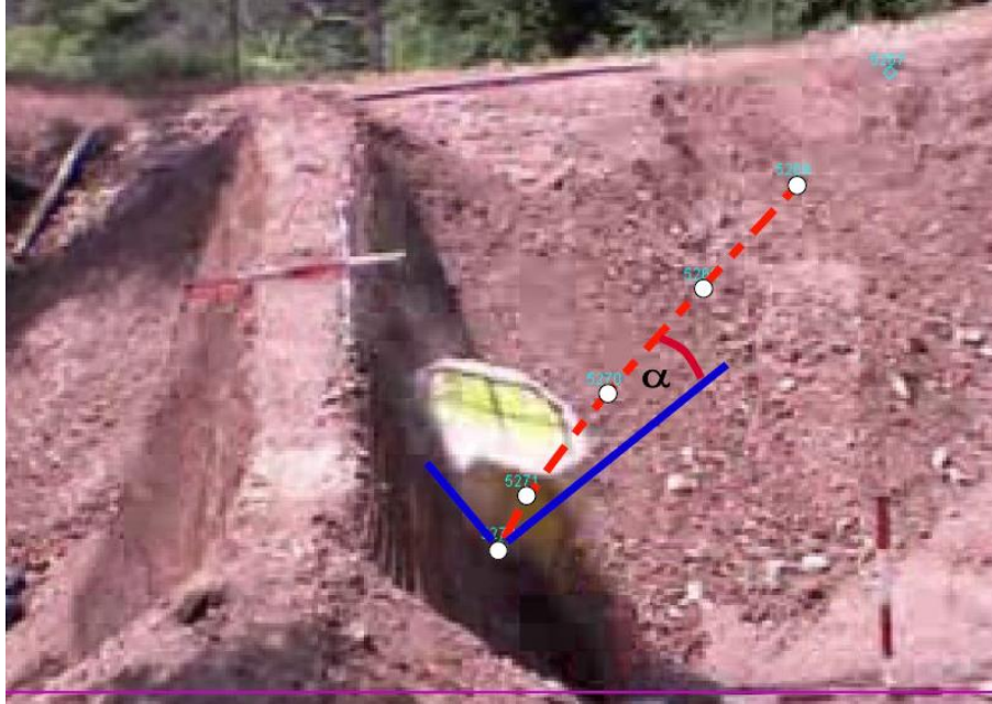
Fig. 4.11: Full size test done by Peila et al. (2007). Result of an analysis with the program Tracker of a movie presented by Tenax Geosynthetics. The test shows a negative impact angle.
