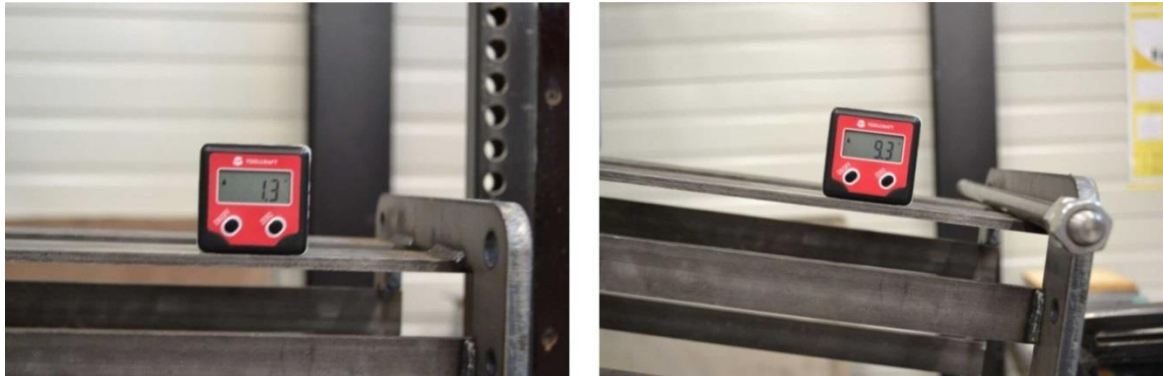
Fig. 2.3: Inclinations of the down pipe exit used in the tests.
