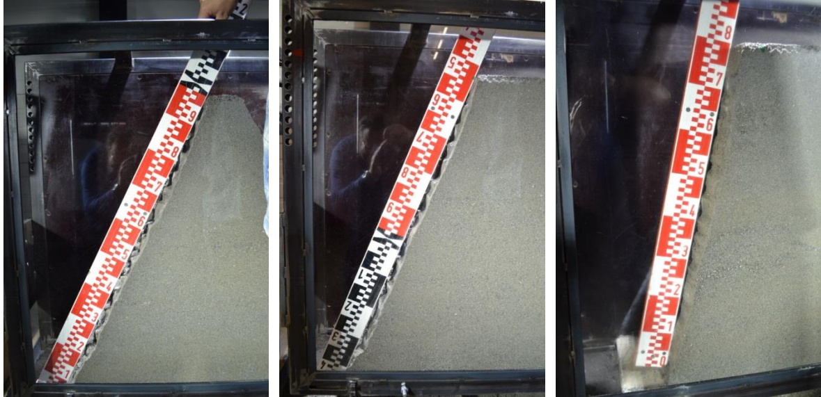
Fig. 2.17: Roughness of the “rockery” with masonry stones placed horizontally for slopes with batter 2:1, 5:2 and 5:1. The roughness is reduced with increase of slope steepness.
