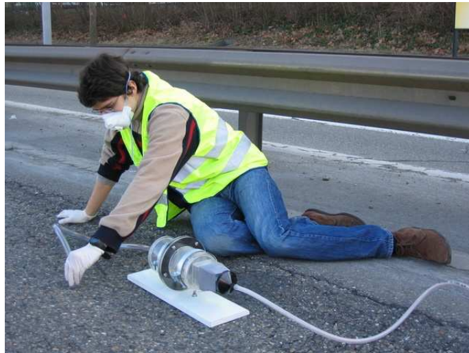
Fig. 3.12: PM10 sampling at Pfingstweidstrasse in Zürich.
