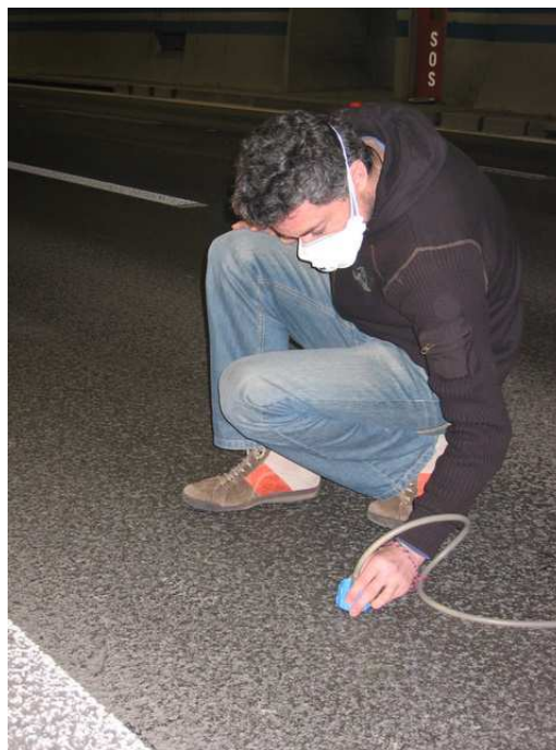
Fig. 3.13: Coarse dust sampling in the Milchbuck tunnel.
