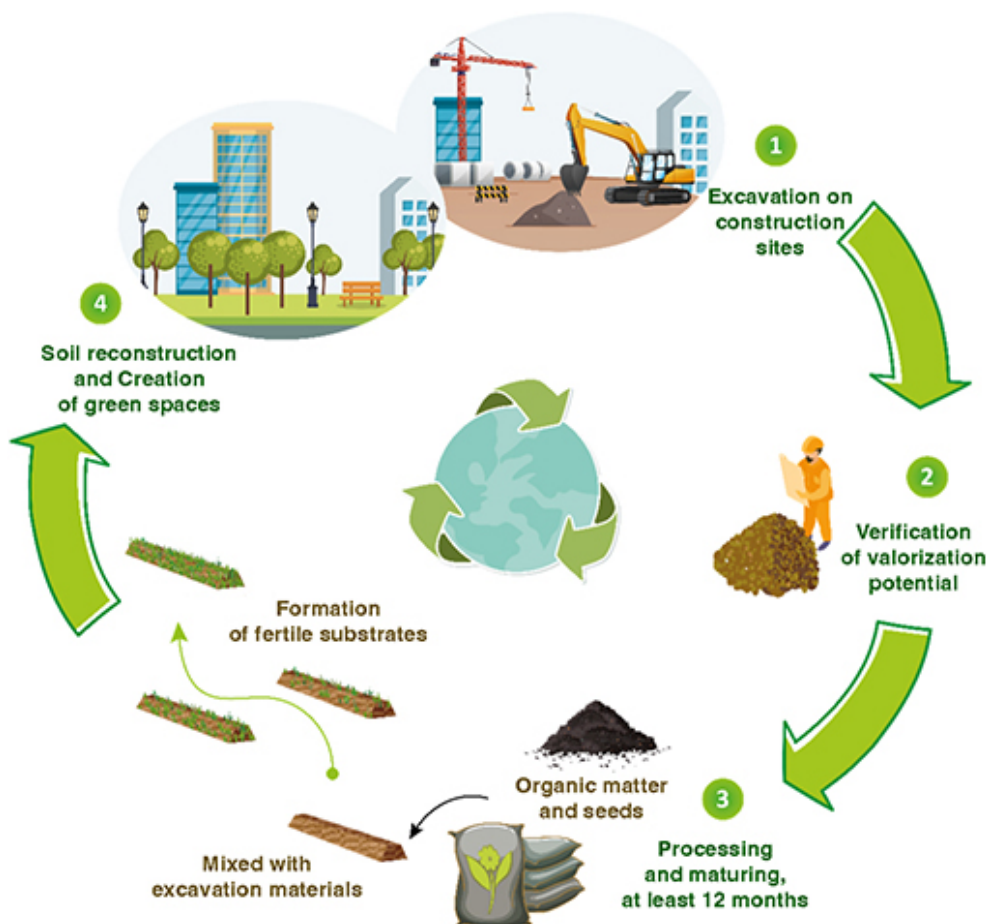
Fig. 19: Diagram of the steps involved in recycling excavated material to create fertile substrates.
