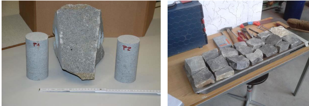
Fig. 2.9: Left: Block of Guber-Quarzsandstein and specimens P1 and P2, which had been used for uniaxial compression test, right: Selected pieces of Guber-Quarzsandstein before placed in the model embankment.
