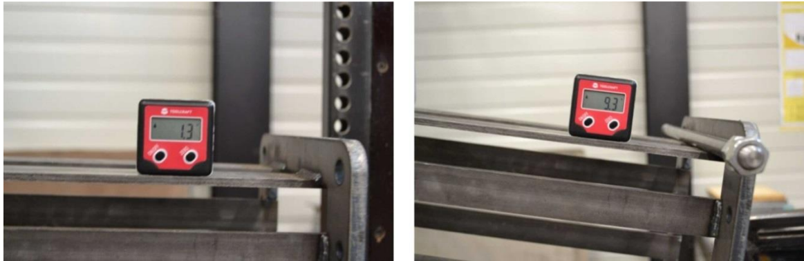
Fig. 2.3: Inclinations of the down pipe exit used in the tests.
