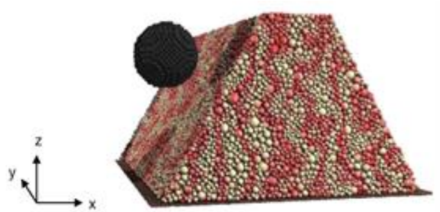
Figure 31 DEM model of embankment and block, both made of “glued” spheres (Plassiard and Donzé, 2010)
