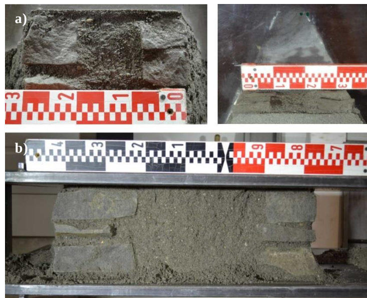
Fig. 2.16: Proportion of stone and soil layer in horizontal sections: a) at the upper third of the embankment, b) at the bottom of the embankment.
