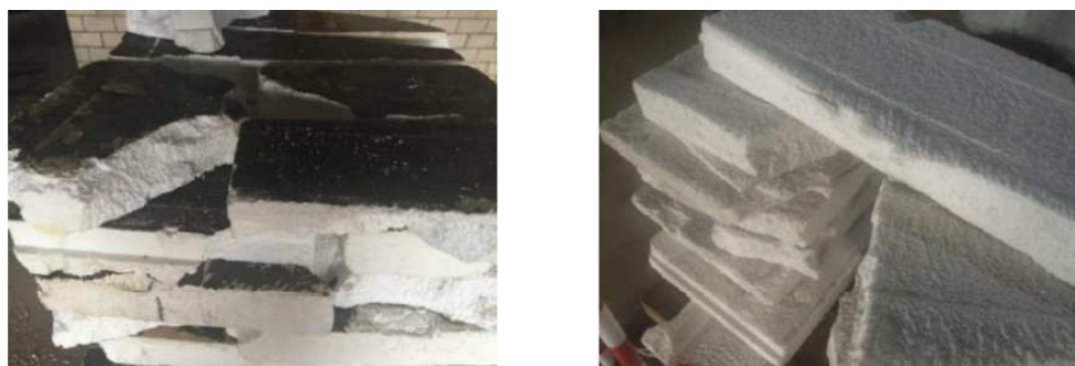
Figure 3. EPS flat roof boards with bitumen leftovers before and after treatment [18].
